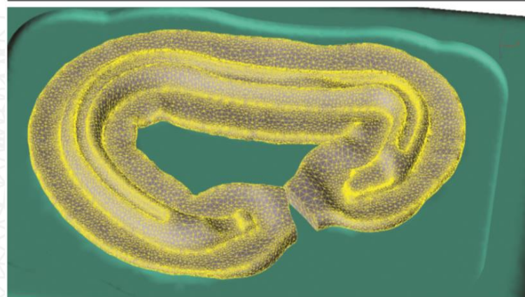
The finite element mesh of an aluminum carabiner forging at the end of stroke.
